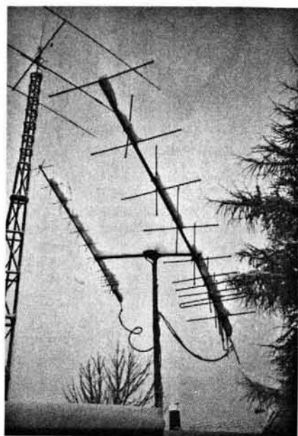
A "Christmas card" scene of the G3IOR satellite antenna system for 144 and 430MHz, well detuned by snow
